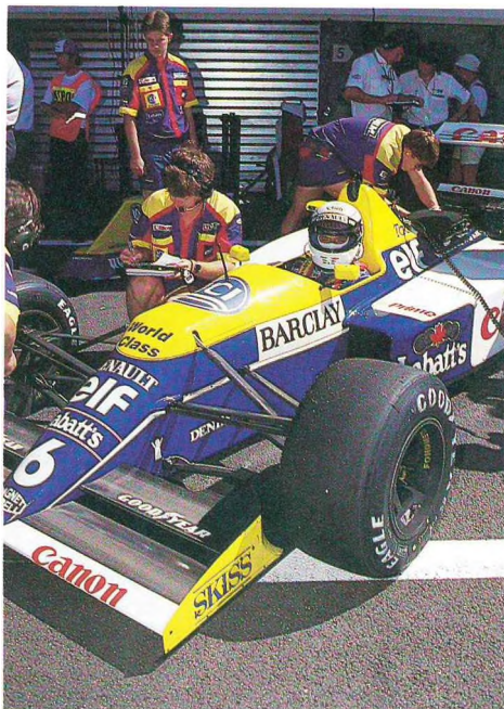
No more "horns"! The Williams FW13 practised with a new Benetton-style nose housing an experimental single shock-absorber front suspension system.
